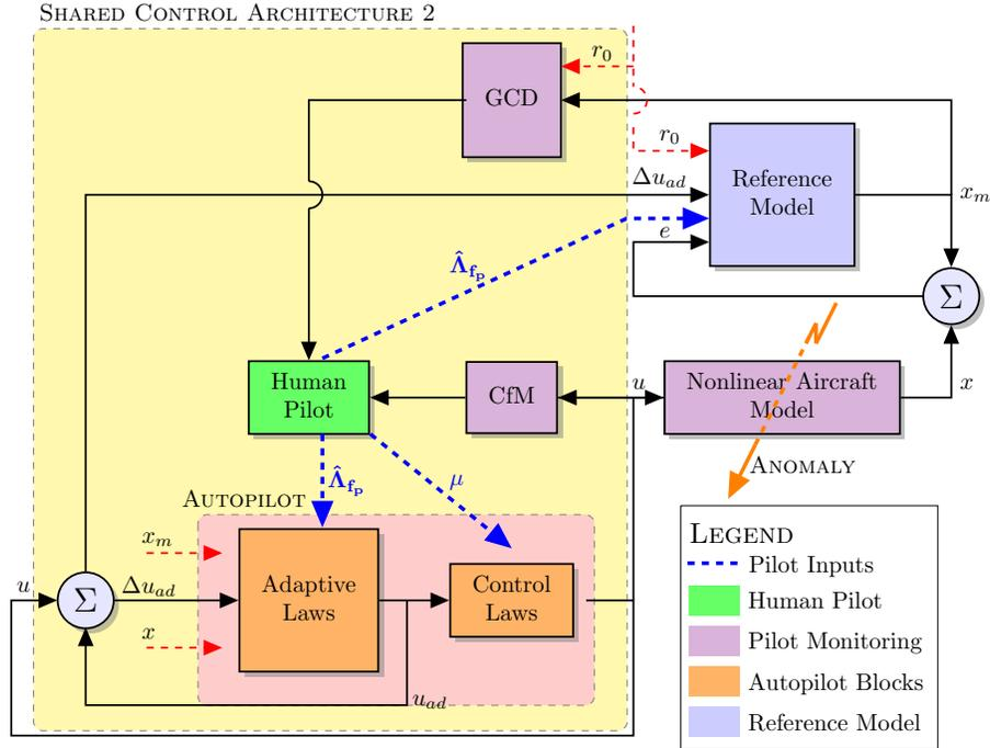
Figure 2: Block diagram of SCA 2. The human pilot undertakes a supervisory role by providing the key parameters  $\mu$  and  $\hat{\lambda}_{fp}$  to the adaptive autopilot. The blocks are expressed in different colors based on their functions in the proposed SCA2.
