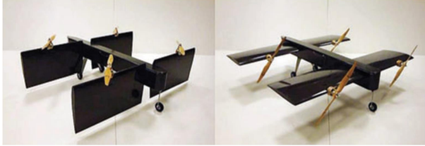
Fig. 1: Quad tilt-wing UAV SUAVI with two different wing angle configurations
